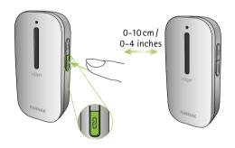
The indicator lights of both microphones will turn green for two seconds to confirm a successful connection.
